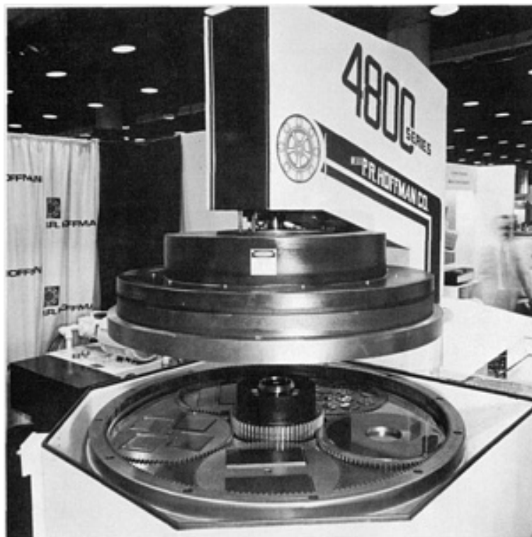
Fig. 3 A 1220 mm (48 in.) planetary top plate drive dual-face lapping machine loaded with a variety of components having various configurations and thicknesses to demonstrate the processing capabilities of the equipment. Shown clockwise, starting with the bottom-most carriers, are hardened high-carbon steel shear blades; 102 by 102 mm (4 by 4 in.) photomask blanks used to project microcircuits onto electronic substrates; stainless steel sender bars, which will be etched into optical position indicators; valve plates machined from cutoff hot-rolled bar stock for use in hydraulic motors; and a hardened alloy steel rotary slit blade.
