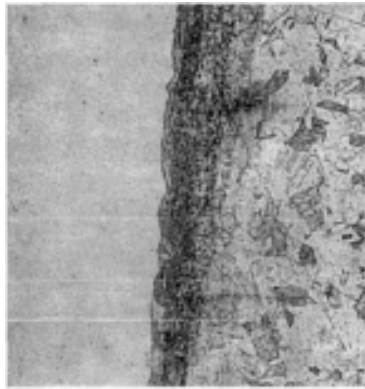
Fig. 4 Etching of 70-30 brass reveals smeared layer
