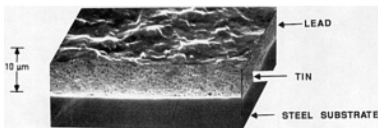
Fig. 16 Terne coating microstructure. Scanning electron microscope cross section
