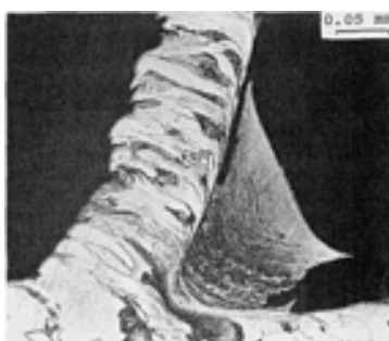
Fig. 7 A chip root obtained when machining 1018 steel with an indexable drill shows the presence of a builtup edge at a speed of 70 m/min (230 ft/min). Source: Ref 15
