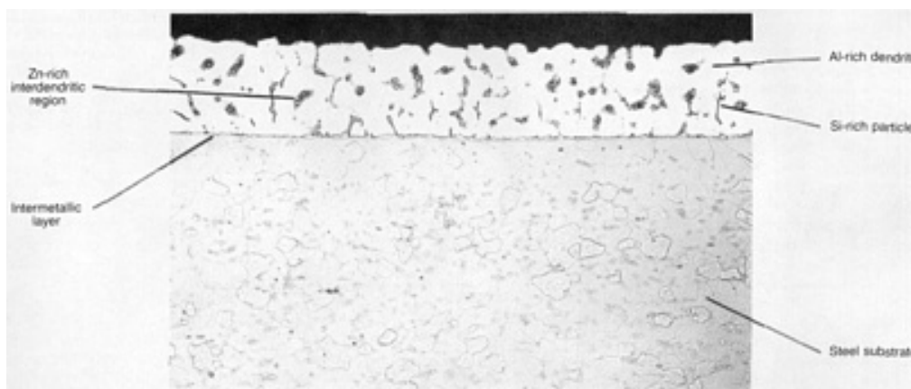
Fig. 12 Microstructure of an aluminum-zinc coated sheet
